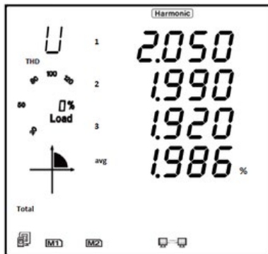
Figure 3-25 Harmonic Distortion Reading
