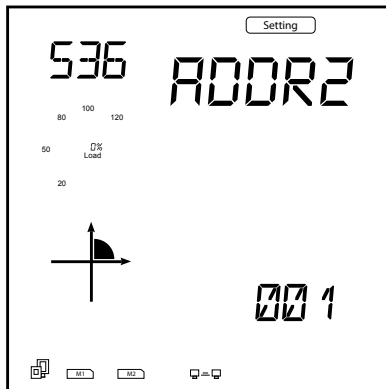
Figure 5-56 Address Setting for AXM-RS485
