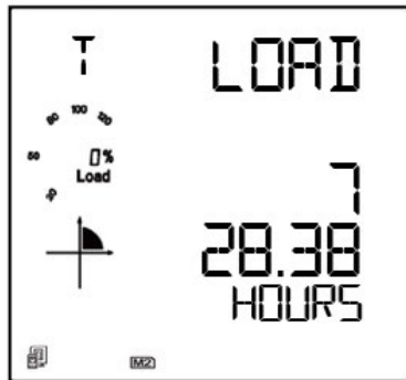
Figure 3-16 Load Time Display
