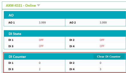
Figure 5-26 Pulse Counter Readings from the Acuvier 2 Software
