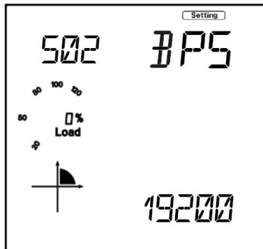
Figure 6-3 System Parameter Setting - S02 Baud Rate
