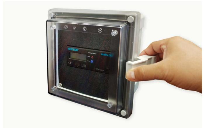
Screws are provided to secure the hinged lid. Local codes may require this step to prevent opening by unauthorized persons if a locking mechanism is not used. For added security, the installer may also add a locking mechanism.
