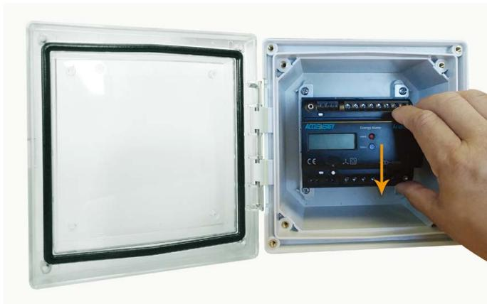
Push the bottom of the meter onto the DIN rail until there is an audible click.
