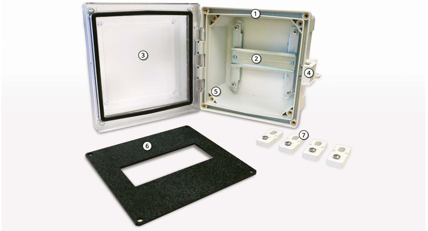
The **AcuRev1310 enclosure** offers a mounting option for AcuRev1310 Series energy meters that helps protect from tampering and the elements. The enclosure is equipped with DIN rail mounting hardware for easy installation, and a NEMA®4X rating ensures durability. The swing panel kit and multiple locking options provide additional security from unwanted tampering.
