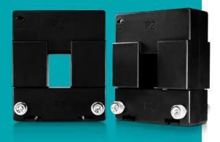
The AcuCT 5A Series is a rugged, compact split-core current transformer designed with an either 1A or 5A industrial output. Choose from multiple sizes & input ranges to adapt to a variety of special project requirements. The helpful split-core design is easy to install and does not require disconnection of cables or wires.
