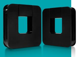
Ideal for gathering high-precision measurements in commercial or industrial electrical panels or switchgear, the AcuCT mV Series is a revenue grade current transformer with a safe, 333mV output. The AcuCT mV is compatible with a range of meters or other instrumentation and the pull-apart, split-core design helps facilitate fast installation without cable or wire disconnection.
